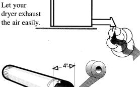
Use 4 inch diameter rigid metal duct. Tape all joints. Never use lint-trapping screws.
